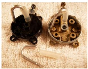
The replacement pick up tube is bent from 3/32" O.D. soft aluminium tubing & chamfered at the bottom to fix exactly. Silicone tubing attaches it to the tank back.
