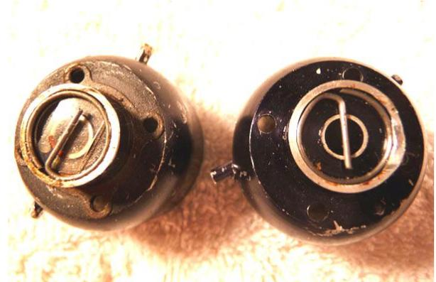
Black Widow tanks: note severe wear around reed retaining 'G-clip' area and reed seal venturi hole area.
