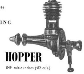
THE Thermal-Hopper came in for test with quite a reputation behind it. In the first place it is a novelty from the design point of view in employing crankcase induction controlled by a reed valve. In the second place quite fantastic r.p.m. figures are claimed by the manufacturers and, thirdly, it is claimed as the fastest starting engine in its class. Like the majority of American production engines it has glow plug ignition.
