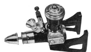
Moulded engine mounts, made by L. M. Cox for the Tee Dee .049 convert it to a firewall radial mounting as seen in above view
