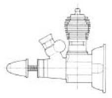
little .010. For example, the engine was found to be capable of turning a  $4^{1}/_{2}$ in x 3 TopFlite wood prop but this loaded it down to a mere 10,800 r.p.m. The .010 is obviously at its best when lightly loaded for speeds in excess of 20,000 and we found it to be capable of running smoothly and steadily at over 30,000 r.p.m.
